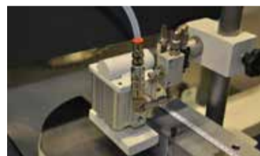
Vertical pneumatic clamps
