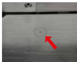
Air jets in the table bed create an air film between the timber and the table for a better through feed.
