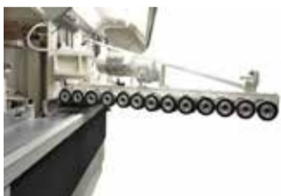
The feeding device has 13 wear resistant wheels. Every wheel is separately spring-loaded.
